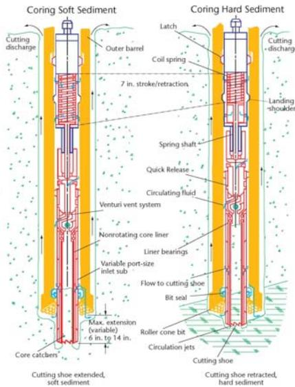
**Schematic of the XCB retractable cutting shoe in standard coring mode. The XCB shoe extends 6 to 14 in. ahead of the bit in very soft formations and retracts ~7 in. (inside the main bit) as weight on bit exceeds about 12,000 lb (collapses a coil spring).**
