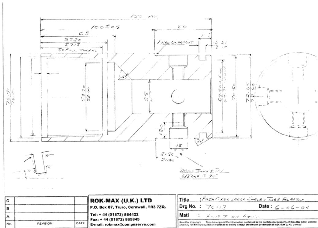
**Shelby Tube Adaptor as fitted to BGS ECB Marine Wireline Coring System (3" variety shown.)**
