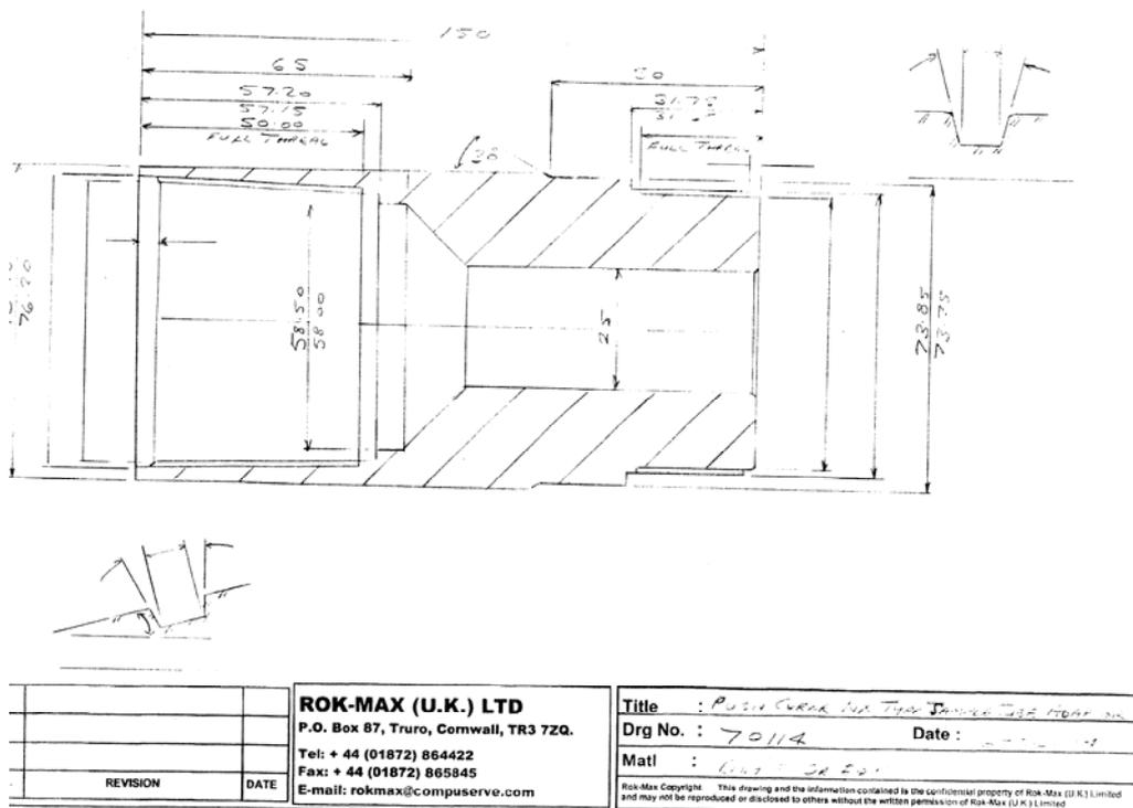
**Push Sampler Adaptor as fitted to BGS ECB Marine Wireline Coring System**
