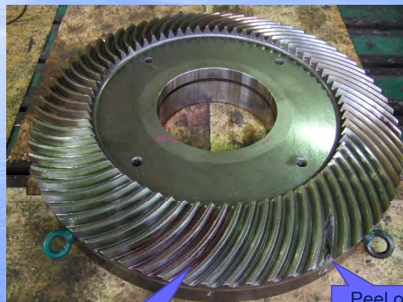
Damage on Wheel of 4S Thruster
