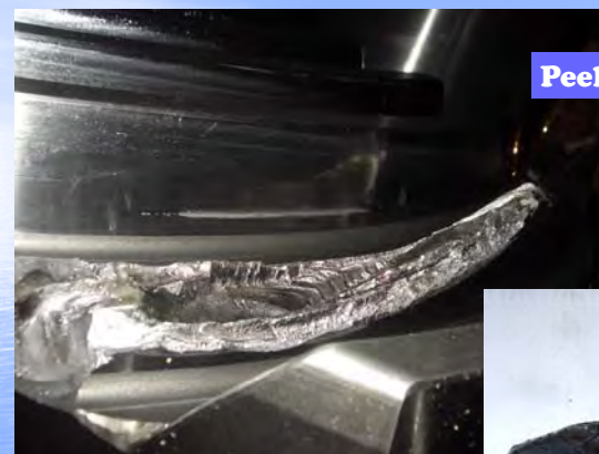
Detail of Damage on Wheel of 4S Thruster
