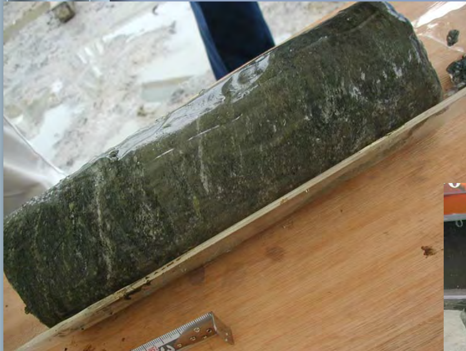
Recovered core without Anti-contamination gel
