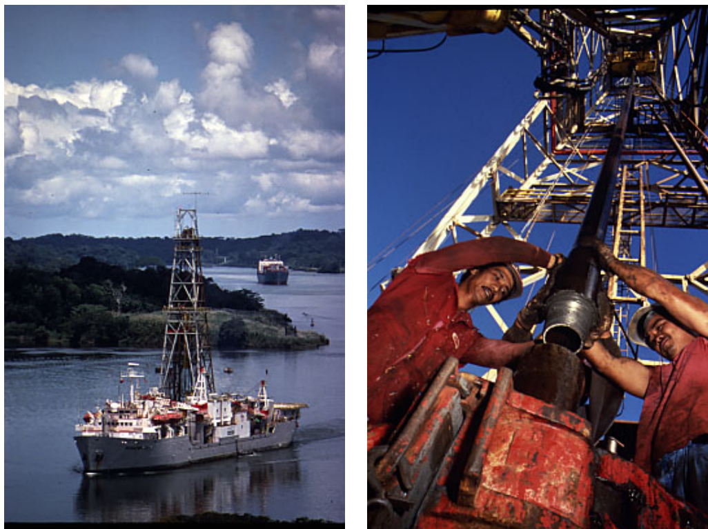
Fig. 4: JOIDES Resolution. (Left) JOIDES Resolution was converted in Pascagoula, Mississippi, in the fall of 1984. She was built in Halifax, Nova Scotia in 1978 and had previously sailed the world as a top-class oil-exploration vessel. (Right) The ship can deploy up to 30,000 feet of drill string.
