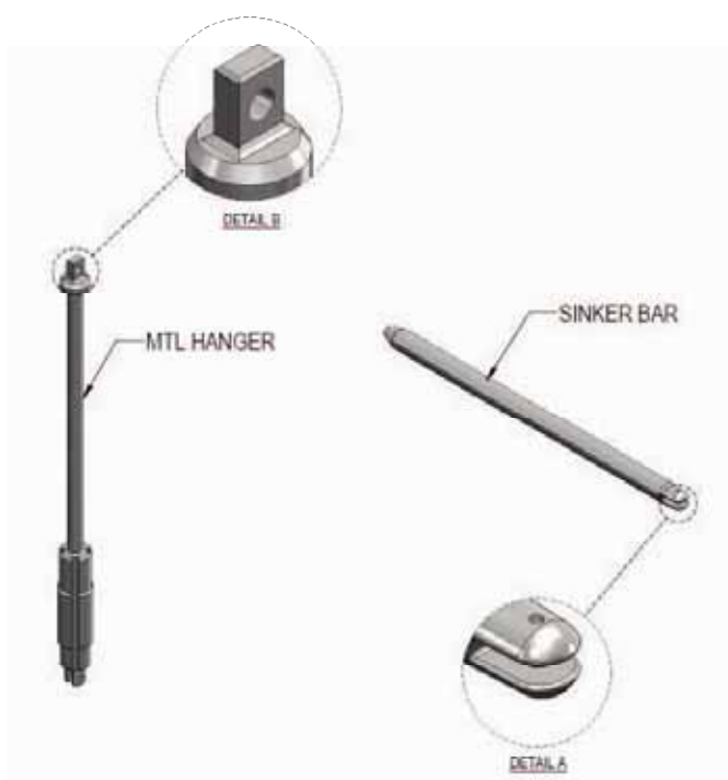
Figure 33. MTL hanger and sinker bar.
