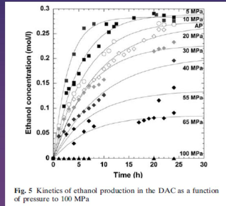
Fig. 5 Kinetics of ethanol production in the DAC as a function of pressure to 100 MPa
