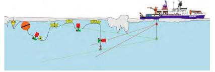
Most instrument deployments are dependant on partly open water within ice cover.
